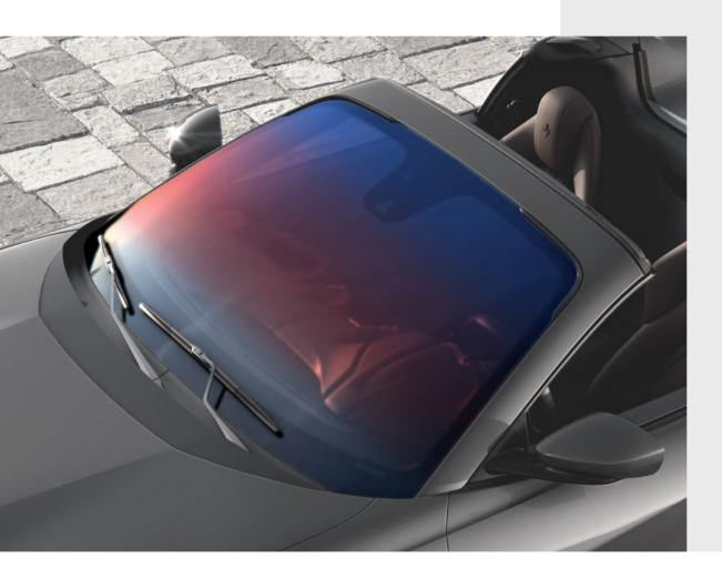
Ferrari offers a completely transparent athermic windshield in place of the conventional windshield.
