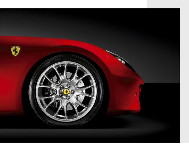
The single-piece 14-spoke wheels, cast in aluminum alloy, enhance the sports concept of the vehicle. Available in a wide range of colors, the 20" Challenge style wheels also come with a special shiny ball-polished finish which enhances its shapes and forms.
