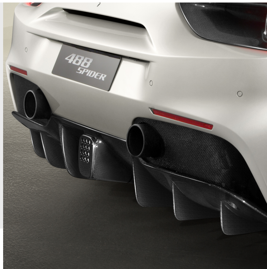
Carbon fiber rear fog light bezel, with analogue camera
