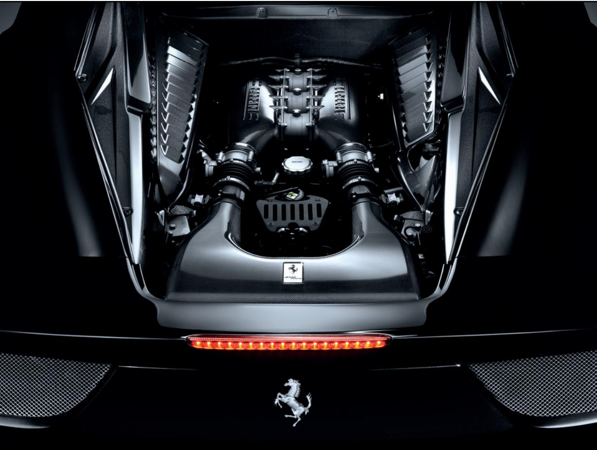
The carbon fiber engine compartment shields are lighter than the standard parts. Carbon fiber is an ultralight, heat resistant material that is also durable thanks to its technical and aesthetic properties and the clear protective layer that covers it.
