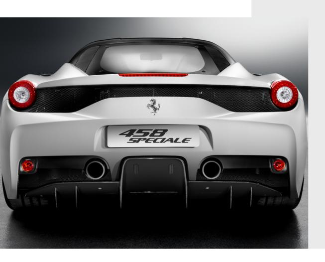
The carbon fiber aerodynamic flaps make a strong aesthetic impact and help to reduce the vehicle's overall weight.
