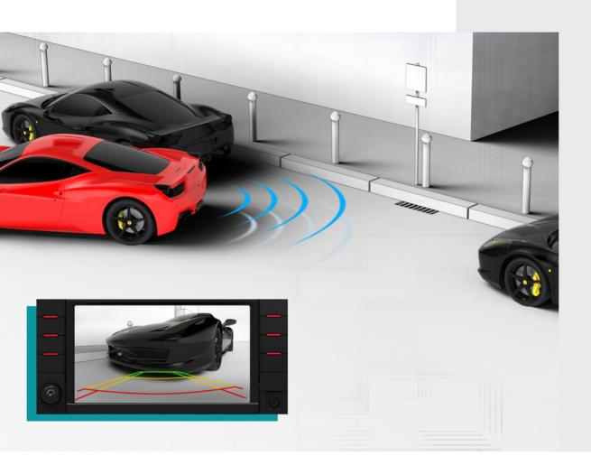
The Ferrari parking camera system helps to prevent accidentally hitting an obstacle when parking. The kits, which include front and rear cameras, display the necessary information on the instrument panel and, thanks to the addition of parking sensors and a practical virtual grid, assist the driver when maneuvering
