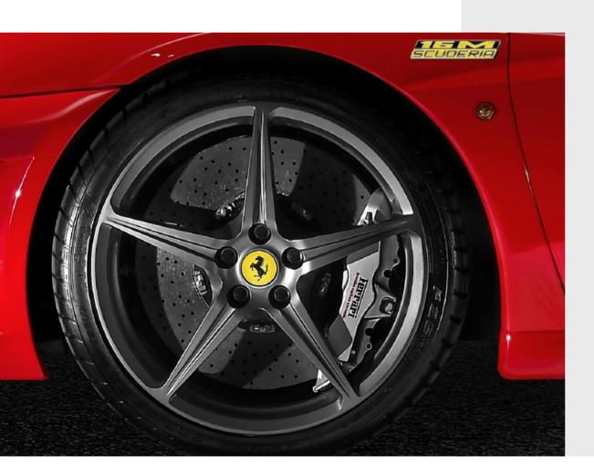
Using forged wheels reduces the weight by 11 kg compared with standard wheels. A reduction in non-suspended mass guarantees a more direct feeling of contact with the vehicle, allowing customers with a more dynamic and demanding driving style to fully enjoy the sports spirit of their car.
